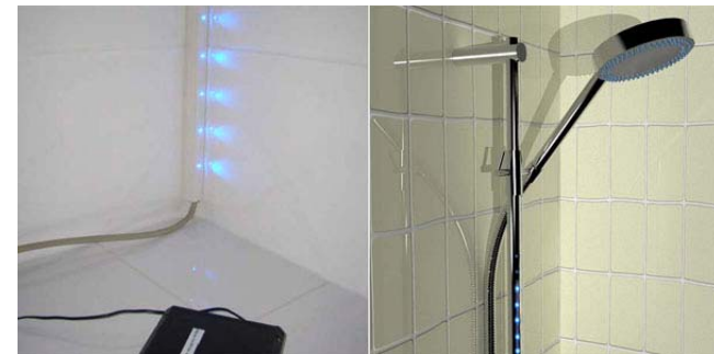
Figure 1. LED-bar prototype of Show-me (left) and a further integrated design solution (right) [11].
