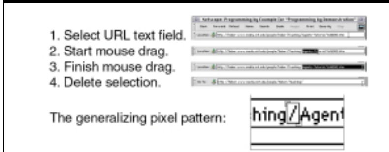
Figure 2. Steps in a mouse macro to move a browser up one directory. And using Triggers to select a pixel pattern that generalizes the macro.
