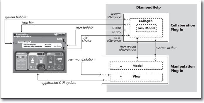
Figure 6. DiamondHelp Software Architecture.
